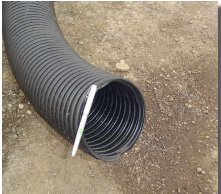
Common flexible polyethylene drainage pipe is plowed below the surface and brought out to the surface on the foreslope at regular intervals to complete this work.
